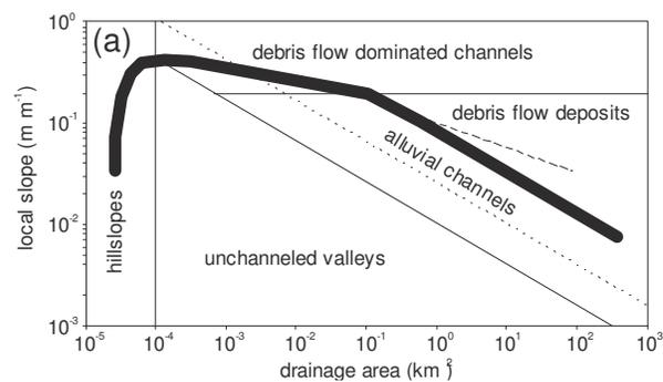
**Figure 1.** Slope-area plot process domains defined by Montgomery and Foufoula-Georgiou [8] and Brardinoni and Hassan [9]. The dotted line indicates the adjustment of the fluvial regime for martian gravity.
