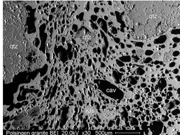
**Fig. 2:** Backscattered electron image of the biotite granite (thin section); qtz: (ballen) quartz, Kfs: K-feldspar, cav: cavity/vesicle (see also Fig. 1).
