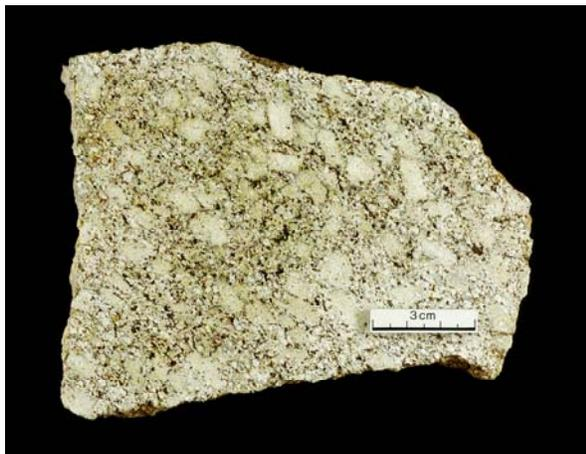
**Fig. 1:** Polished section of the partially molten biotite granite (clast in melt rock) recovered from the Polsingen quarry, Nördlinger Ries; bright domains are *in situ* molten and recrystallized K-feldspars.
