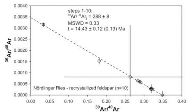
**Fig. 4:** Inverse isochron plot; all steps (black circles) are included in the plateau fraction; errors as cross symbols; uncertainties are at the 1  $\delta$  level; error in parentheses includes the error of the age standard.
