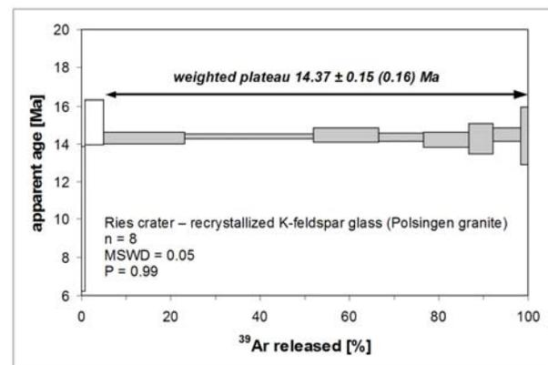
**Fig. 3:**  $^{40}\text{Ar}/^{39}\text{Ar}$  age spectrum for recrystallized potassium feldspar glass separate from partially molten biotite granite (Polsingen, Nördlinger Ries); uncertainties are at the 1  $\delta$  level; error in parentheses includes the error of the age standard.
