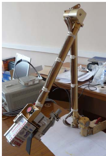
Fig 2. MIMOS II sensorhead mounted on the robotic arm.
