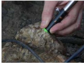
Figure 3: Raman at other spots in the outcrop detected pure goethite.
