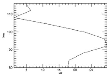
**Figure 3:** Limb profile of the c-X (0-8) band, integrated over the 0.48-0.50  $\mu\text{m}$  range. The vertical resolution was smoothed, to avoid spurious features. The maximum of the emission is observed at about 95 km height as obtained with a Gaussian curve fit. The FWHM is about 16 km.
