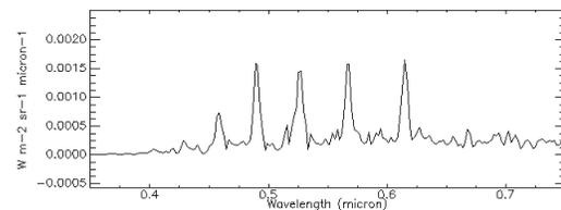
**Figure 1:** VIRTIS-M spectrum, obtained by averaging about 1300 spectra, acquired on 30 October 2009 in the limb view mode. The Herzberg II progression is clearly visible, with transitions centred at 0.46  $\mu\text{m}$ , 0.49  $\mu\text{m}$ , 0.52  $\mu\text{m}$ , 0.57  $\mu\text{m}$  and 0.61  $\mu\text{m}$ .
