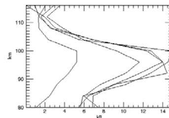
**Figure 2:** Limb profile of the (0-7), (0-8), (0-9), (0-10) and (0-11) c-X bands. The vertical resolution was smoothed, to avoid spurious features. The maximum of the emission is observed at about 96 km.
