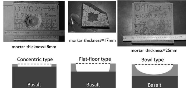
**Figure 1:** Crater type formed on the basalt target covered with mortar
