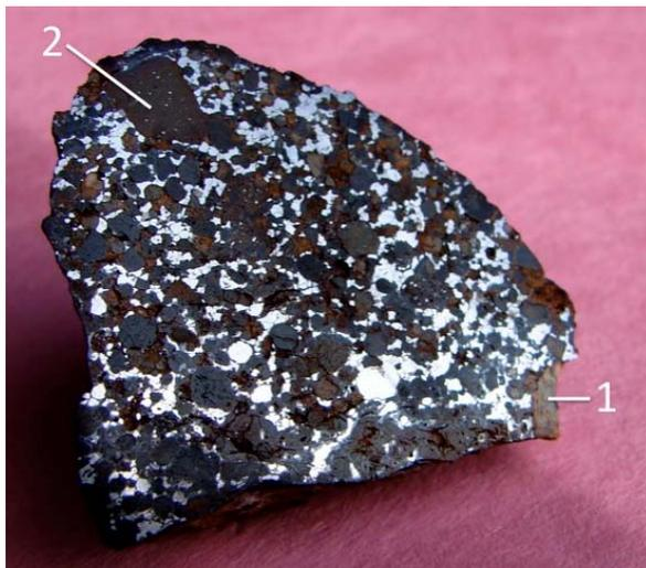
**Figure 1.** Cut surface of NWA 5492 showing metal nodules (white), chondrules and angular lithic fragments. Oxygen isotope compositions were determined for objects labeled 1 and 2.
