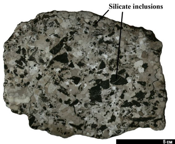
Fig.1. Macroscopic image of etched polished slice of the NWA 6369 iron.
