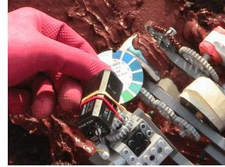
Fig. 6. On site comparison of the standard and the ribbon color in an extraordinary sunlight condition at Kamond.
