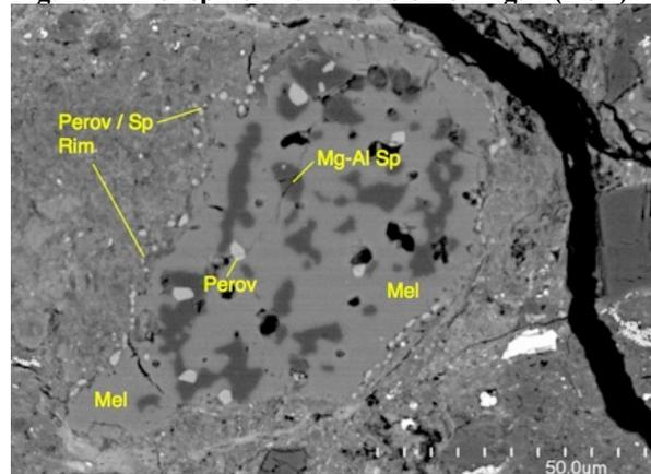
**Fig. 3:** BSE image of a melilite-rich CAI in MET 00426, 46. It shows inclusions of Mg-Al spinel and perovskite within melilite, but also a very fine-grained perovskite and Mg-Al spinel rim.
