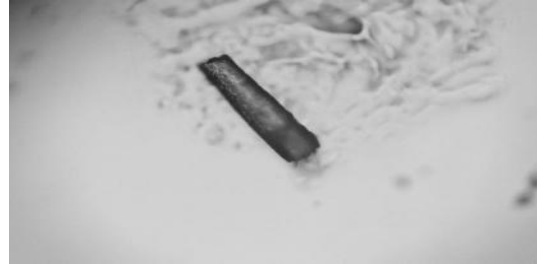
Fig. 3A. Extracted cylinder (60 \mu\text{m} in diameter) from apatite crystal containing inclusion.
