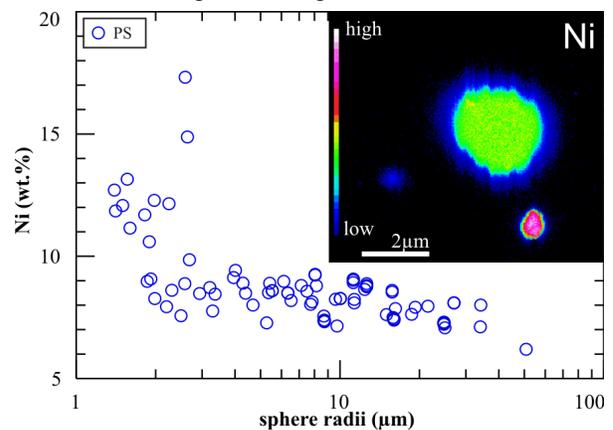
**Fig. 5.** Ni-content vs. sphere radii; insert shows a Ni element map.; for legend see Fig. 2.
