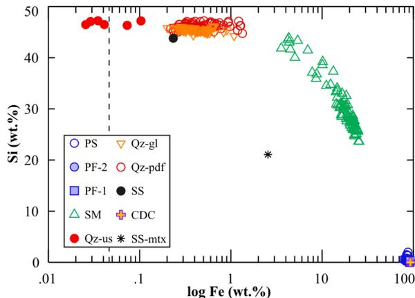
**Fig. 2.** Fe vs. Si for various materials of Exp. # 3298.; PS: projectile sphere; PF-1: partly fused projectile fragment; PF-2: projectile fragment; SM: sandstone melt; Qz-un: unshocked quartz; Qz-gl: quartz glass; PDF: PDFs in quartz; SS: Seeberger sandstone; CDC: Campo del Cielo projectile; SS-mtx: mean of the sandstone matrix. Dashed line corresponds to the average detection limit for Fe.
