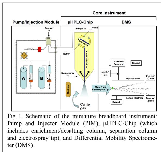
Fig 1. Schematic of the miniature breadboard instrument: Pump and Injector Module (PIM),  $\mu$ HPLC-Chip (which includes enrichment/desalting column, separation column and electro-spray tip), and Differential Mobility Spectrometer (DMS).
