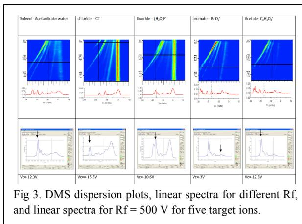
Fig 3. DMS dispersion plots, linear spectra for different Rf, and linear spectra for Rf = 500 V for five target ions.
