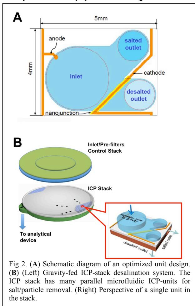
Fig 2. (A) Schematic diagram of an optimized unit design. (B) (Left) Gravity-fed ICP-stack desalination system. The ICP stack has many parallel microfluidic ICP-units for salt/particle removal. (Right) Perspective of a single unit in the stack.
