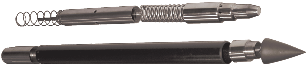
Fig 1. The laboratory model of the mole penetrator: casing with the tip (bottom) and the hammer with the support (top)
