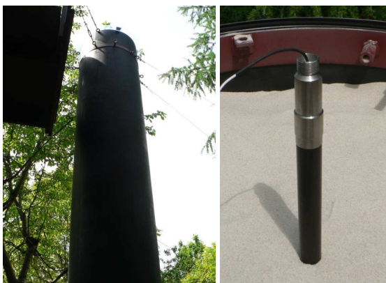
Fig. 4. The 5-m test-bed (left) and the mole KRET in the test-bed before commencing the test (right).
