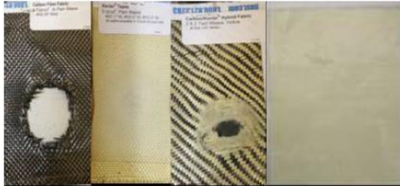
Figure 2: Carbon Fiber (A), Kevlar (B), Hybrid (C), and Vectra (D) textiles after exposure to lunar simulant spray.
