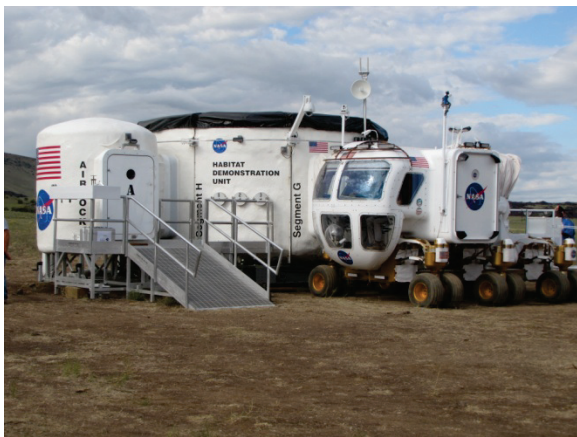
Figure 1: SEV rover docked to HDU1-PEM. The image also shows the three GeoLab glovebox pass-through antechambers and EVA porch (center).
