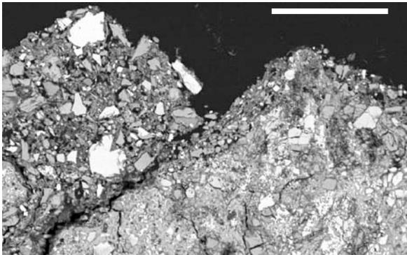
**Fig. 5** BSE image of a particle with a fine-grain ash size core surrounded by a rim that is much thicker on the left. The rim consists of subrounded ash-size ilmenite, plagioclase and augite fragments. Rim max clast size 100  $\mu\text{m}$ . Scale bar  $\sim 250 \mu\text{m}$ .
