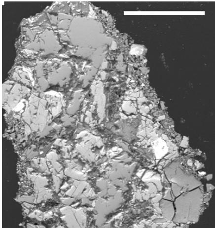
**Fig. 2** (left) BSE image showing a shocked basaltic core with fine-grain, rim composed of mineral fragments. Max particle size in rim 25  $\mu\text{m}$ . Scale bar ~250  $\mu\text{m}$ .
