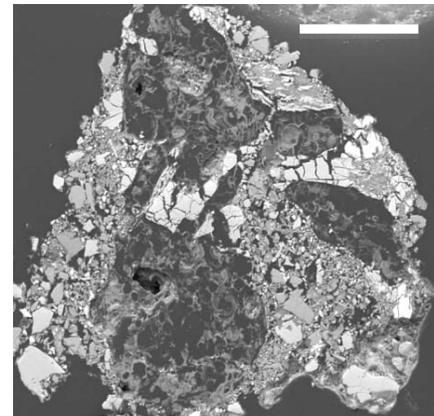
**Fig. 4** (right) BSE image showing a shocked mineral core (bottom), topped with a zone of melted material high in feldspar component and a fine-grain rim. Max clast size for melt and rim is 50  $\mu\text{m}$ . Scale bar ~250  $\mu\text{m}$ .
