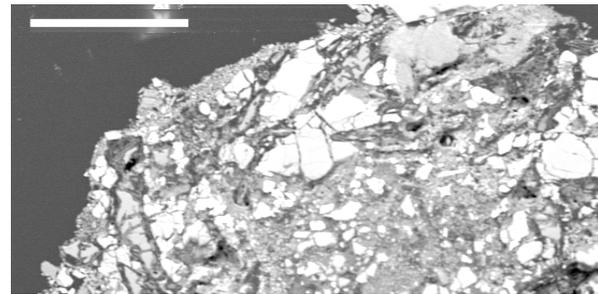
**Fig. 6** BSE image of a particle consisting of a conglomerate of ash size fragments of ilmenite, augite, and glass surrounded by a fine-grain rim of the same composition. Rim max clast size 50  $\mu\text{m}$ . Scale bar  $\sim 250 \mu\text{m}$ .
