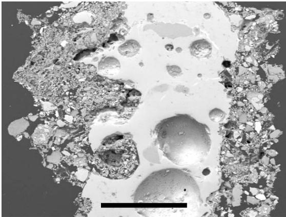
**Fig. 1** BSE image of a vesicular, impact melt core with a fine-grain rim composed of mineral grains and scoriaceous melt. Max particle size in rim ~50  $\mu\text{m}$ . Scale bar ~250  $\mu\text{m}$ .
