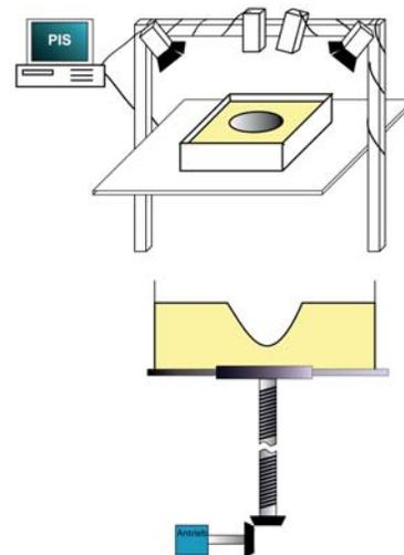
Fig. 1 Experimental set-up. A piston beneath the box moves at constant velocity and causes instabilities of the cavity in the granular medium. Two cameras film the movements of flank wall collapse of a paraboloid cavity.
