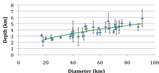
**Figure 3.** Depth-diameter relationship for 43 of the 45 craters in our initial study. Two craters with diameters in the range 100 to 110 km are excluded as they are shallow (depths  $< 5$  km) relative to the rest of the population.
