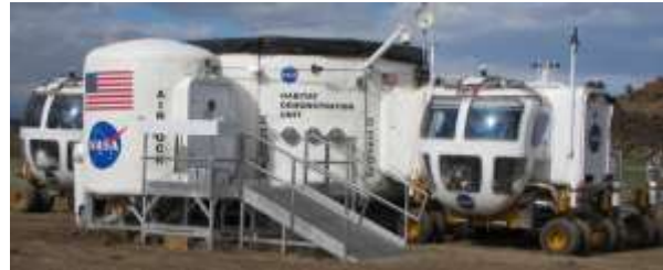
Figure 2: The HDU1-PEM with two rovers docked. The three circular ports directly below "Habitat Demonstration Unit" are the antechamber doors that provide access directly into the GeoLab Glovebox.
