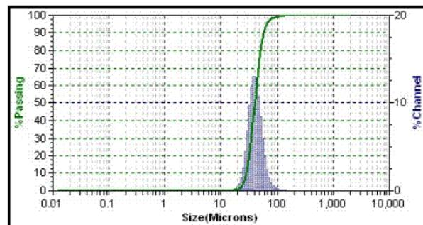
Figure 2c. Microtrac results for 20-45 μm sieve fraction.
