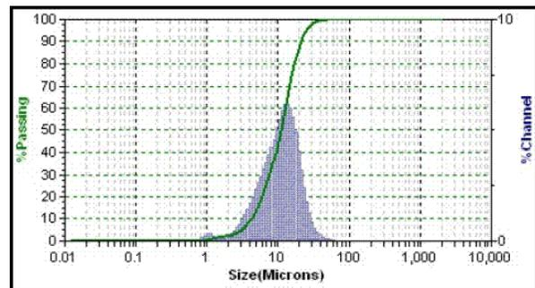
Figure 2d. Microtrac results for <20 μm sieve fraction.
