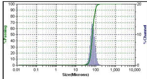
Figure 2b. Microtrac results for 45-75 μm sieve fraction.
