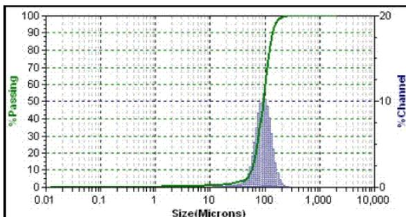
Figure 2a. Microtrac results for 75- 90 μm sieve fraction.
