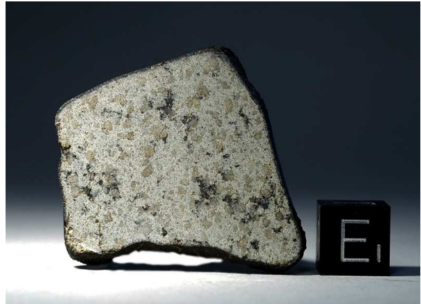
Figure 2 (above). Endcut fragment, showing yellow-green olivine grains in a pale beige pigeonite-rich groundmass. Shock glass pockets are black. Scale cube is 1 cm. Photo © S. Ralew.
