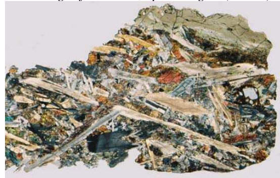
Figure 3b (below). Cross-polarized light thin section image of a coarser, ophitic region (13 mm).
