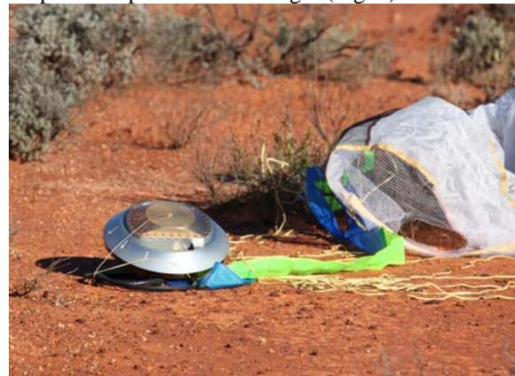
Fig. 1: The re-entry capsule at the landing site before its recovery.
