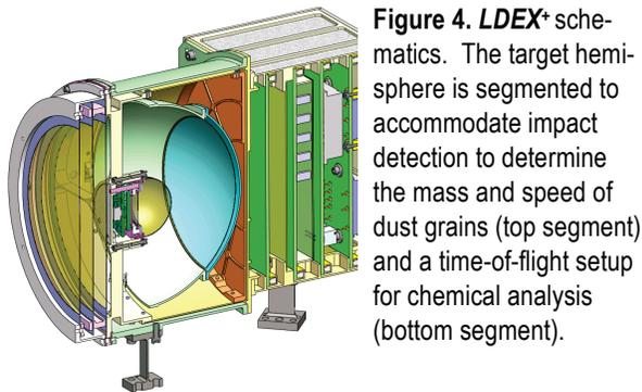
**Figure 4.** *LDEX+* schematics. The target hemisphere is segmented to accommodate impact detection to determine the mass and speed of dust grains (top segment) and a time-of-flight setup for chemical analysis (bottom segment).
