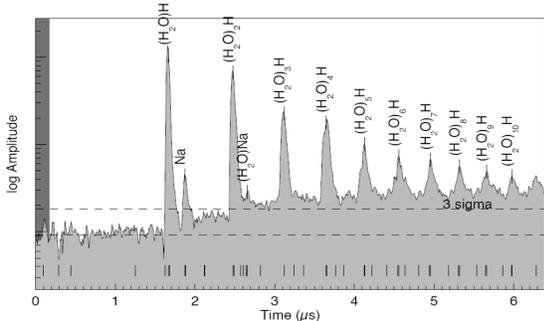
**Figure 5.** Spectrum of a water ice particle obtained at  $\sim 4$  km/s impact speed by the Cassini CDA instrument in Saturn's E ring. The dominant peaks are mass lines of water cluster ions  $(\text{H}_2\text{O})_n\text{H}^+$ , generated upon impact of an ice-bearing particle [6].
