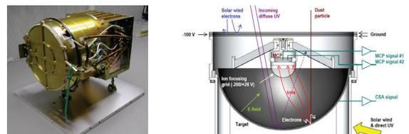
**Figure 2.** Engineering model and schematics of LDEX
