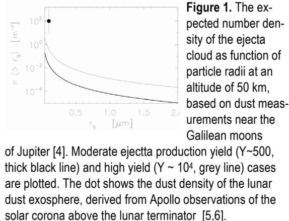
**Figure 1.** The expected number density of the ejecta cloud as function of particle radii at an altitude of 50 km, based on dust measurements near the Galilean moons
