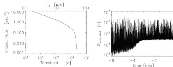
**Figure 3.** The expected impact rate on LDEX from meteoroid impact generated ejecta particles with radii  $r > 0.3 \mu\text{m}$  (left). The expected 'collective' signal from lofted grains during LADEE's approach of the terminator generated by impact of dust grains with radii  $0.1 < r_g < 0.3 \mu\text{m}$  (right).
