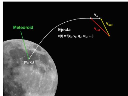
**Figure 6.** Schematics of dust spectrometry of the lunar surface. Ejecta particles lifted by micrometeoroid impacts from the satellites' surface are analyzed by a dust composition mass spectrometer. By tracing the trajectory to the surface, compositional maps of Moon can be generated.
