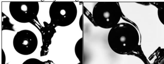
**Figure 3: Ice tendril structures formed during an 11 hour experimental run. The beads are 500-600 $\mu$ m for scale.**
