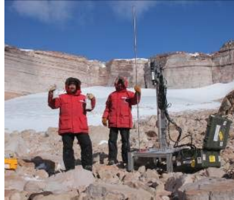
Figure 3. Drilling 2.5 meter in massive ice in the University Valley (the Beacon Valley region of Antarctica.)
