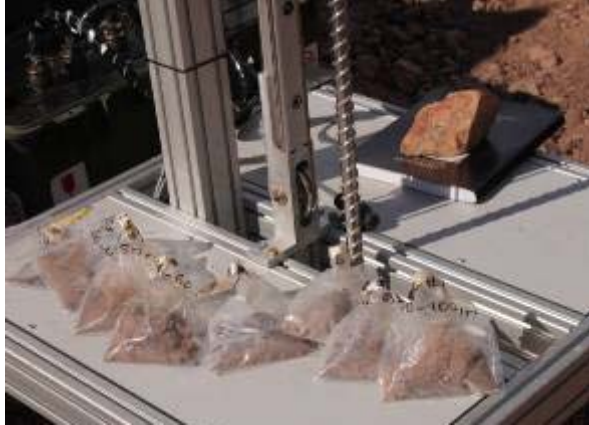
Figure 2. Samples were collected in 10 cm intervals using autonomous sampling system (only replacing of bags after each 10 cm interval was not automated).
