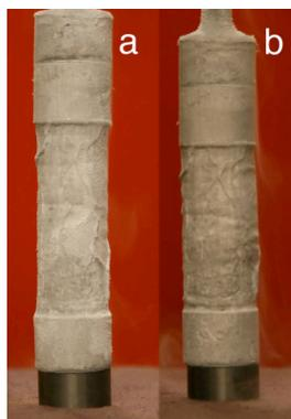
Figure 1. Indium-jacketed polycrystalline ice+perchlorate sample (a) after hydrostatic compaction and (b) after deformation. Right-cylindrical shape indicates a well-behaved experiment. For scale, diameter of column is 25 mm.
