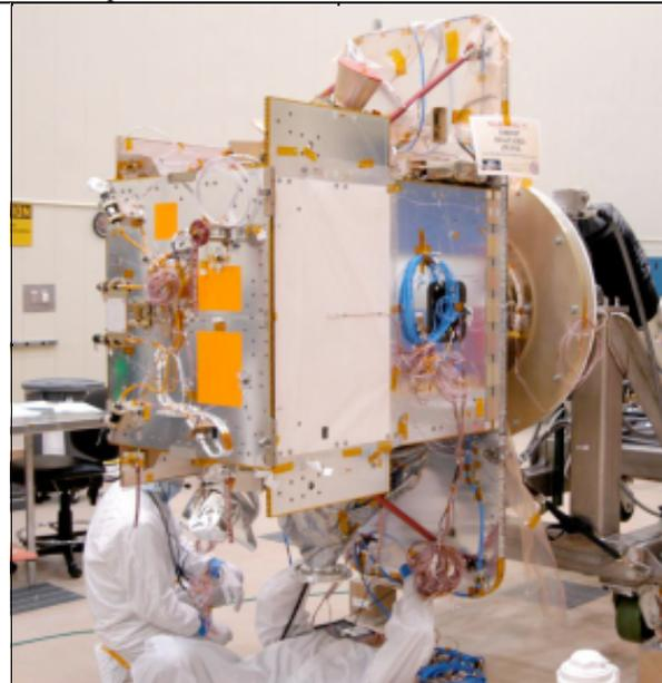
**Figure 2.** Completed GRAIL-A spacecraft bus.
