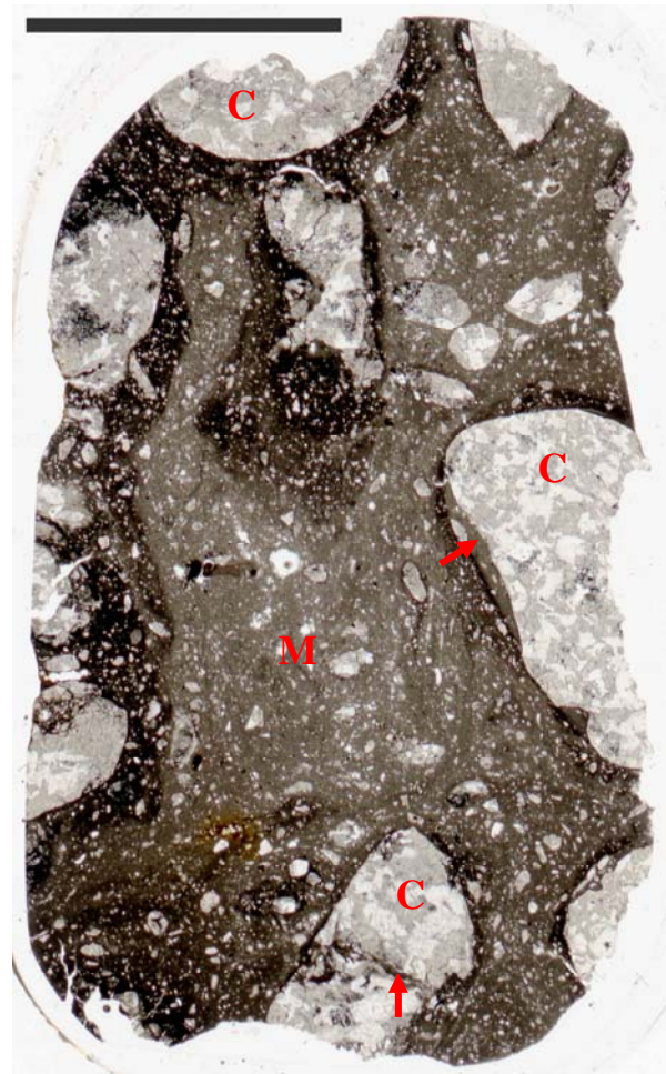
Figure 1. Thin section scan of NWA 5218. Black bar is 1 cm long. C - clast, M - melt; arrows indicate trachytic-textured melts.
