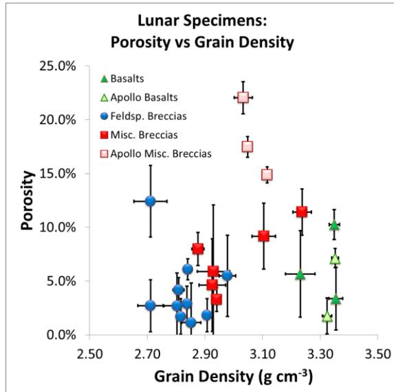
Fig. 2: Porosity vs. Grain Density for lunar specimens in this study. Note that the three Apollo breccias have higher porosities than any of the meteorites.
