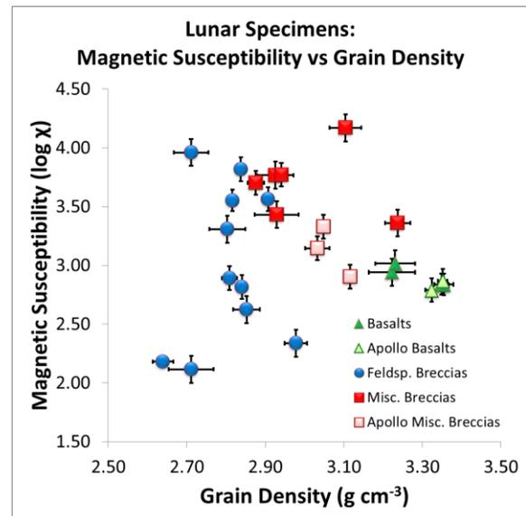
Fig. 1: Grain density vs. magnetic susceptibility for lunar specimens in this study.
