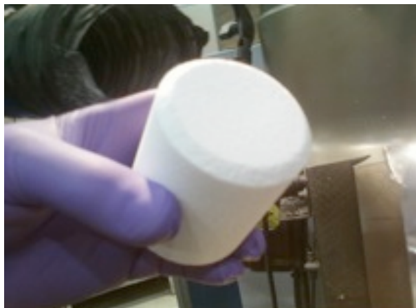
Fig. 2 The OCM bricks have chamfered edges at the top of the cylinder and a positioning groove machined into the base as an anti-rotation feature while drilling. (Photo James Pura).
