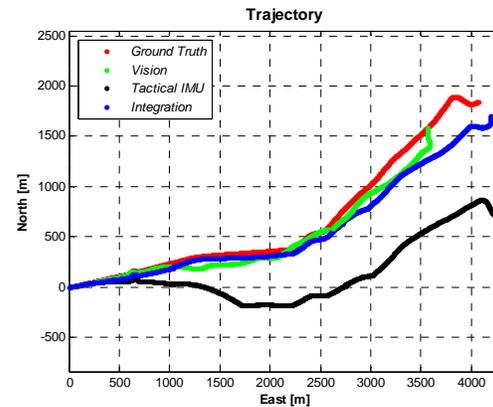
Figure 2. Traverse paths as reconstructed from: LASOIS (blue line), vision sensors (green line), and tactical IMU (black line). Red line represents ground truth.
