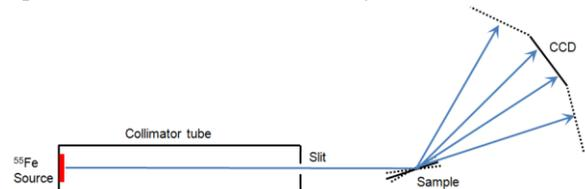
Figure 3 – Schematic diagram of the experimental set-up with both sample and CCD on a rotating axis to replicate incidence/detector angles.
