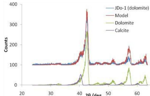
Figure 5 – Dolomite diffractogram (JDo-1, GSJ) model matched to experiment indicating the presence of a calcite component in addition to the main dolomite component.
