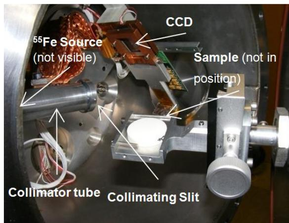
Figure 2 – Experimental set-up of the test facility, Space Research Centre, University of Leicester.
