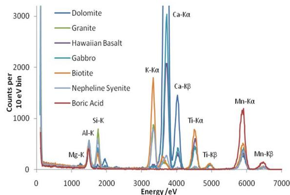
Figure 4 – A selection of Standard Reference Material fluorescence spectra from the highest CCD angle only.
