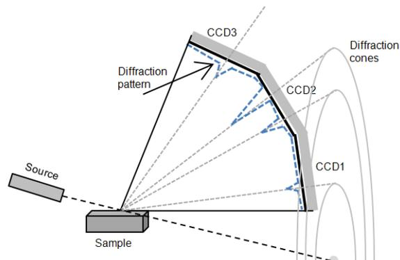
Figure 1 – Mars-XRD measurement concept. CREDIT ESA Mars-XRD Team.
