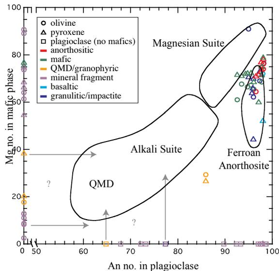
Figure 2. Mg no. ( $100 \times \text{molar Mg}/(\text{Mg}+\text{Fe})$ ) in pyroxene and olivine as a function of An no. ( $100 \times \text{molar Ca}/(\text{Ca}+\text{Na})$ ) in coexisting plagioclase for clasts and mineral fragments.
