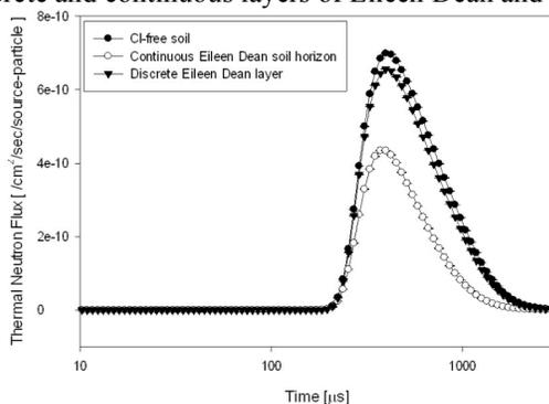
**Figure 2:** Thermal neutron flux as a function of time after the PNG pulse for dry soil composition, as well as a dry soil
