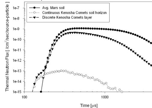
**Figure 3:** Thermal neutron flux as a function of time after the PNG pules for dry soil composition, as well as a discrete layer and continuous layer of Kenosha Comets composition. Data are presented on a log-log plot in order to show all three thermal die-away curves.
