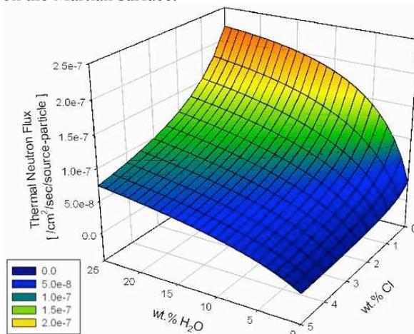
**Figure 1:** Surface plot showing simulated DAN thermal neutron flux as a function of H<sub>2</sub>O and Cl concentration. Legend shows ranges of thermal thermal neutron flux.
