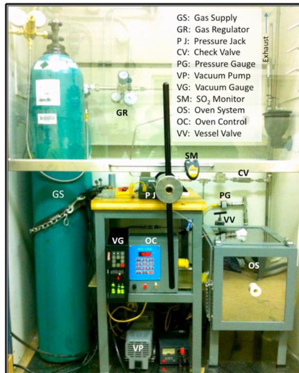
**Figure 1.** A photo of the Venus Weathering System assembled inside a fumehood showing the major components. The high pressure vessel is mounted inside the oven system.
