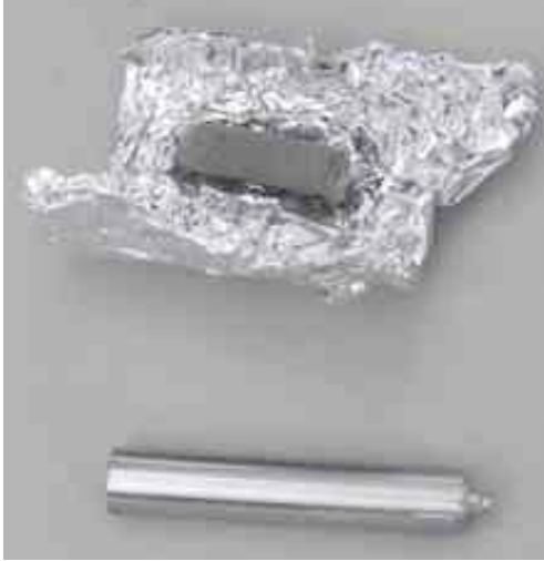
Fig. 3. Sample cache tube and a core. Inner dimensions of the tubes are 1 x 5 cm.
