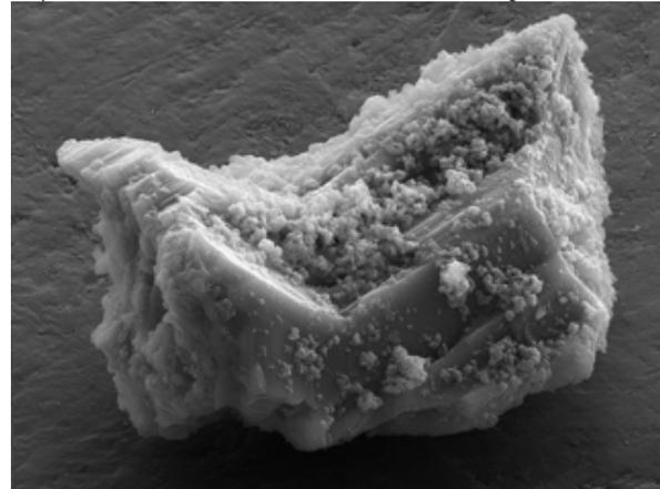
40 $\mu$ m En LSP with growth steps & surface debris
