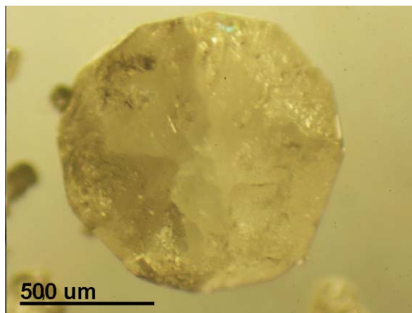
Figure 3. Large (>1mm) synthetic whitlockite crystal produced in a 10 day run.
