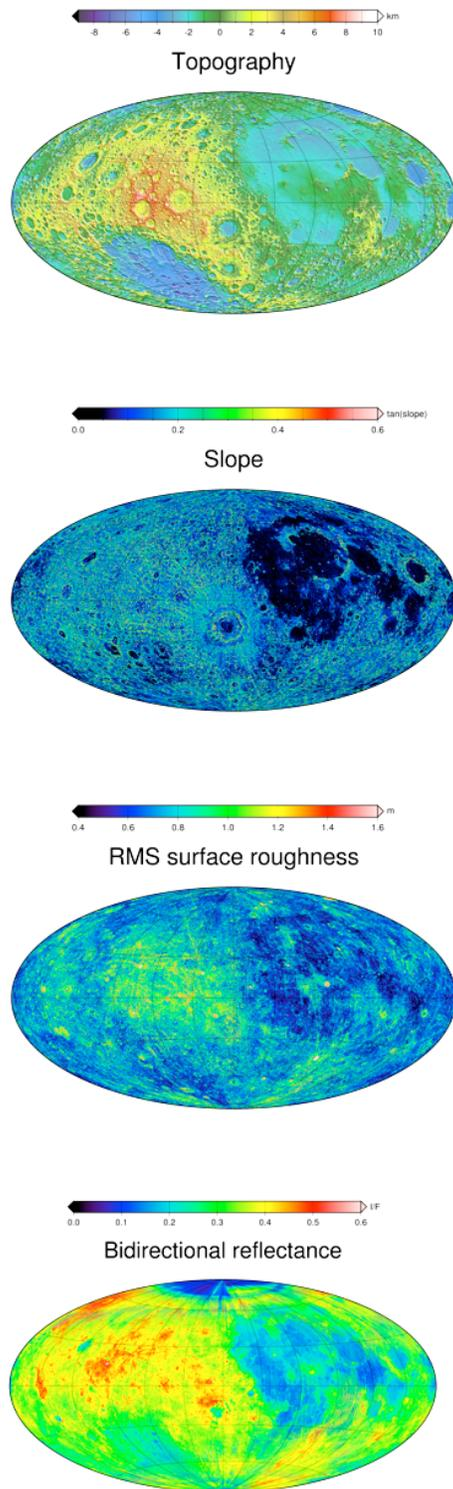
**Figure 1.** Hammer equal-area projections of topography, 56-m-baseline slopes, 5-m-scale rms roughness, and bidirectional reflectance of the Moon as measured by the Lunar Orbiter Laser Alimeter (from [3]).
