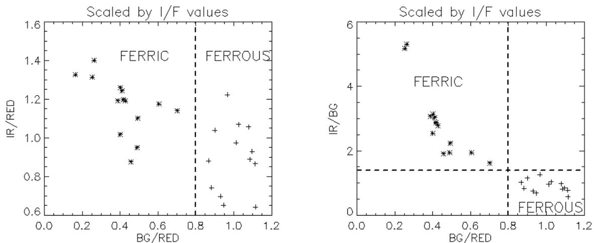
Fig. 1. Band ratio values derived from laboratory mineral, lithologic and surface spectra weighted by the HiRISE spectral response.
