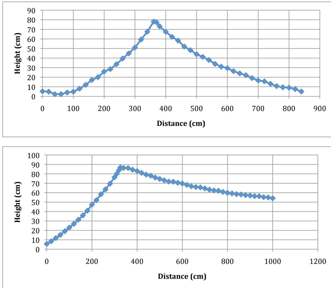
**Figure 2.** Profiles across gravel megaripples at Purulla (upper) and Camp Piedra Pomez (lower). Note the distinct difference in the symmetry of the ripples. At Purulla the ripples show little difference between the lee and stoss sides and are symmetric, while the Campo Piedra Pomez the ripples are clearly asymmetric.
