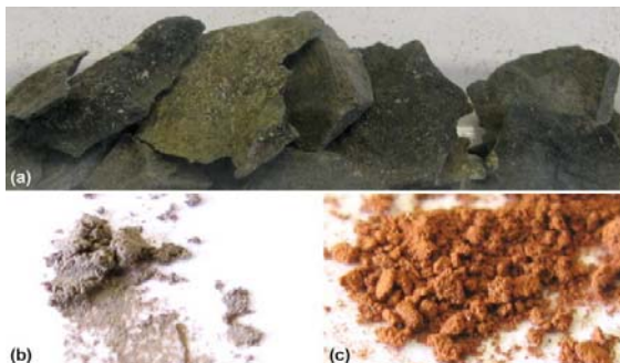
Figure 4 Close-up view of the sample, (a) as collected (image is ~40 mm wide, thus individual shale flakes are ~5 mm across), (b) after grinding in an agate mortar, and (c) after heating to ~ 600 °C in the MOMA oven.
