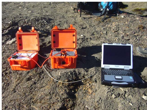
Figure 1 MOMA field equipment deployed at Knorringfjellet, Svalbard, with power supply (left) and one GC (middle).
