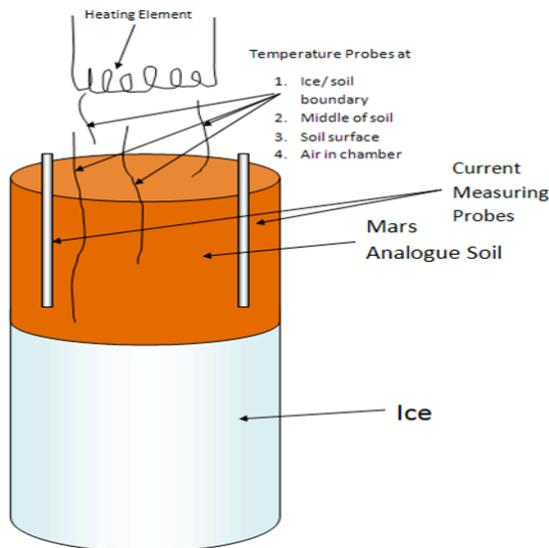
Measurements were performed in the Goddard’s Martian simulation chamber, which allows varying atmospheric pressure, gas composition and temperature of the subsurface ice. Dry JSC-Mars-1 soil analogue was placed on the layer of ice in the vacuum chamber. The surface of the soil was then periodically heated with the heating element to simulate Martian day-night conditions.
