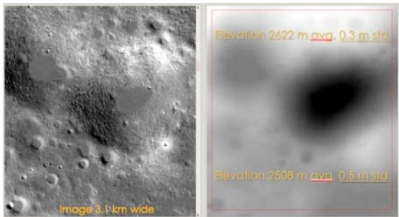
**Figure 2.** LROC NAC stereo image (left) and corresponding derived DEM (right) of small portion of pond region (each 3.1 km wide).
