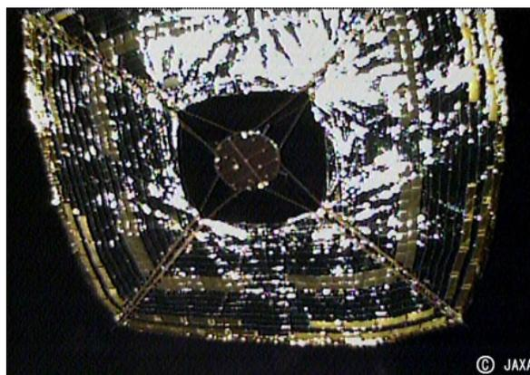
Fig.1 ALADDIN onboard the polyimide membrane of IKAROS solar sail spacecraft (Courtesy: JAXA)
