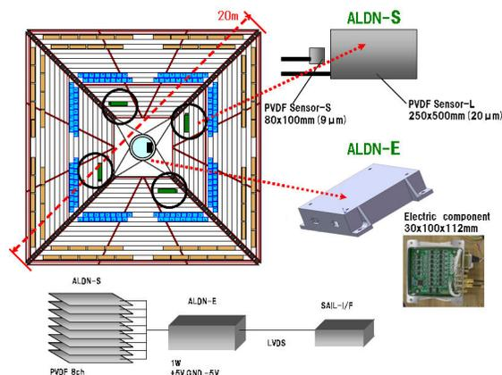
Fig.2 ALADDIN System: all sensors weighed in 39 g and electronic box in 210 g in total
