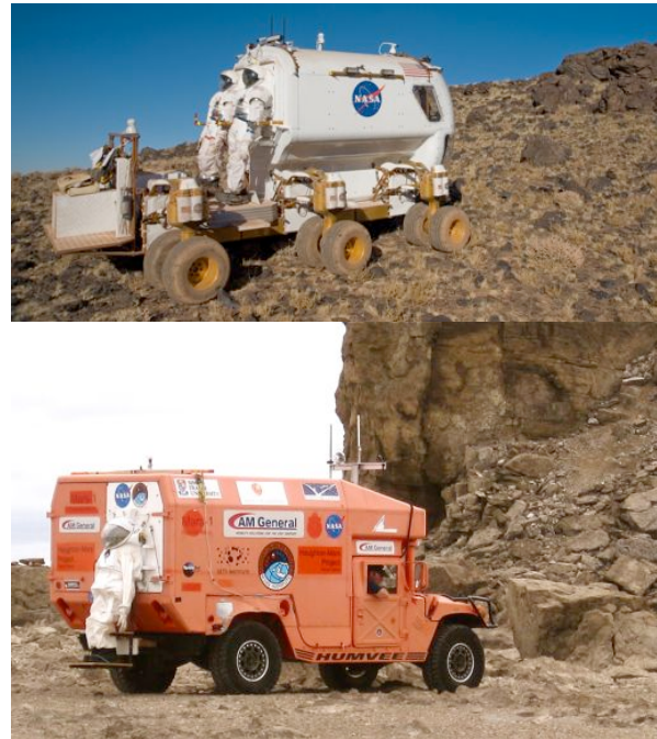
Fig. 1: Top: IVA field science observations from the NASA Lunar Electric Rover during the Desert RATS 2008 analog field campaign. (Photo NASA/DRATS-2008); Bottom: The Haughton-Mars Project's Mars-1 Humvee Rover being used as a pressurized rover analog from which a crewmember conducts field geology in IVA mode. (Photo NASA/Mars Institute/Hamilton Sundstrand/HMP-2009).
