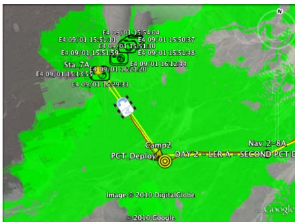
Figure 3. Desert RATS traverse with comm. coverage overlay, vehicle tracks, and geolocated data products.
