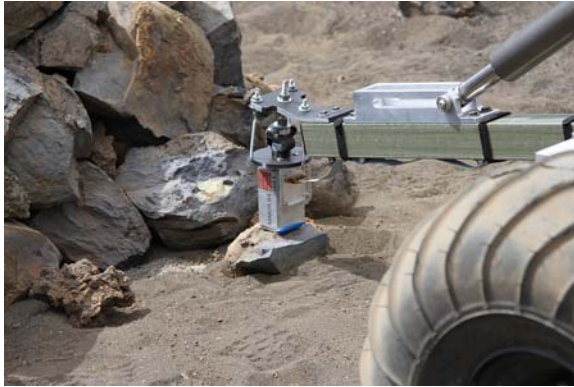
Fig. 3: Combined Mössbauer/XRF-MIMOS IIA mounted on the robotic arm of the NORCAR rover.
